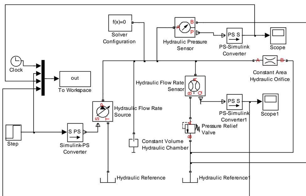
Fig.4. The model consisting of ready-made Simscape items
