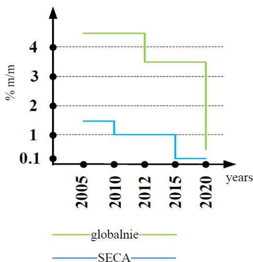
Fig.1. Limits on the sulfur content of marine fuels [1]
