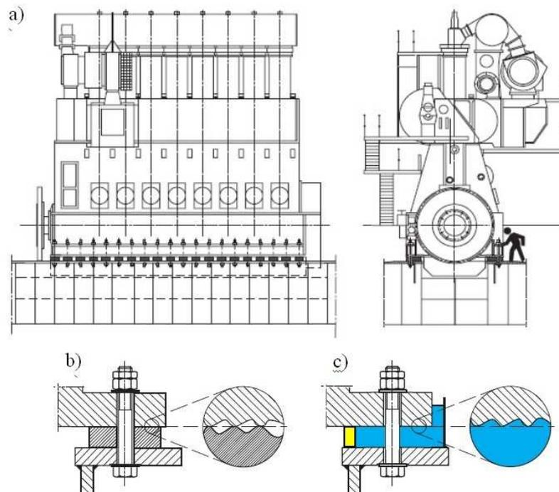
Fig. 1. A schematic of a marine engine seating (a) using chocks made of steel (b) and cast of resin (c)
