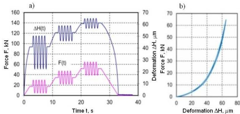
Fig. 7. Time runs of the sinusoidally varying force with a constant amplitude ( $\sigma_m = 3$  MPa) and three different mean values ( $\sigma_a = 4, 8, 12$  MPa) and the deformations caused by it (a); in Fig. b) results of the same measurements in the co-ordinate system  $F - \Delta H$
