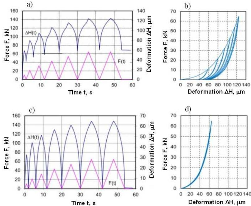
Fig. 3. Time runs of the given compressive loads  $F(t)$  and the deformations  $\Delta H(t)$  caused by them for the first (a, b) and third (c, d) loading cycles (having the same runs); (the maximum values of the surface pressures amounted sequentially to:  $\sigma_1 = 2,5, 5,0, 7,5, 10,0, 12,5$  and  $15,0$  MPa)
