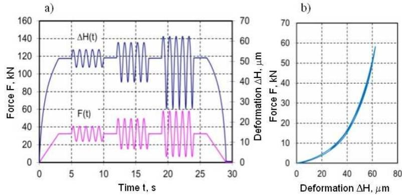
Fig. 6. Time runs of the sinusoidally varying force with a constant mean value ( $\sigma_m = 7.5$  MPa) and three different amplitudes ( $\sigma_a = 2, 4, 6$  MPa) and the deformations caused by it (a); in Fig. b) - results of the same measurements in the co-ordinate system  $F - \Delta H$  (b)
