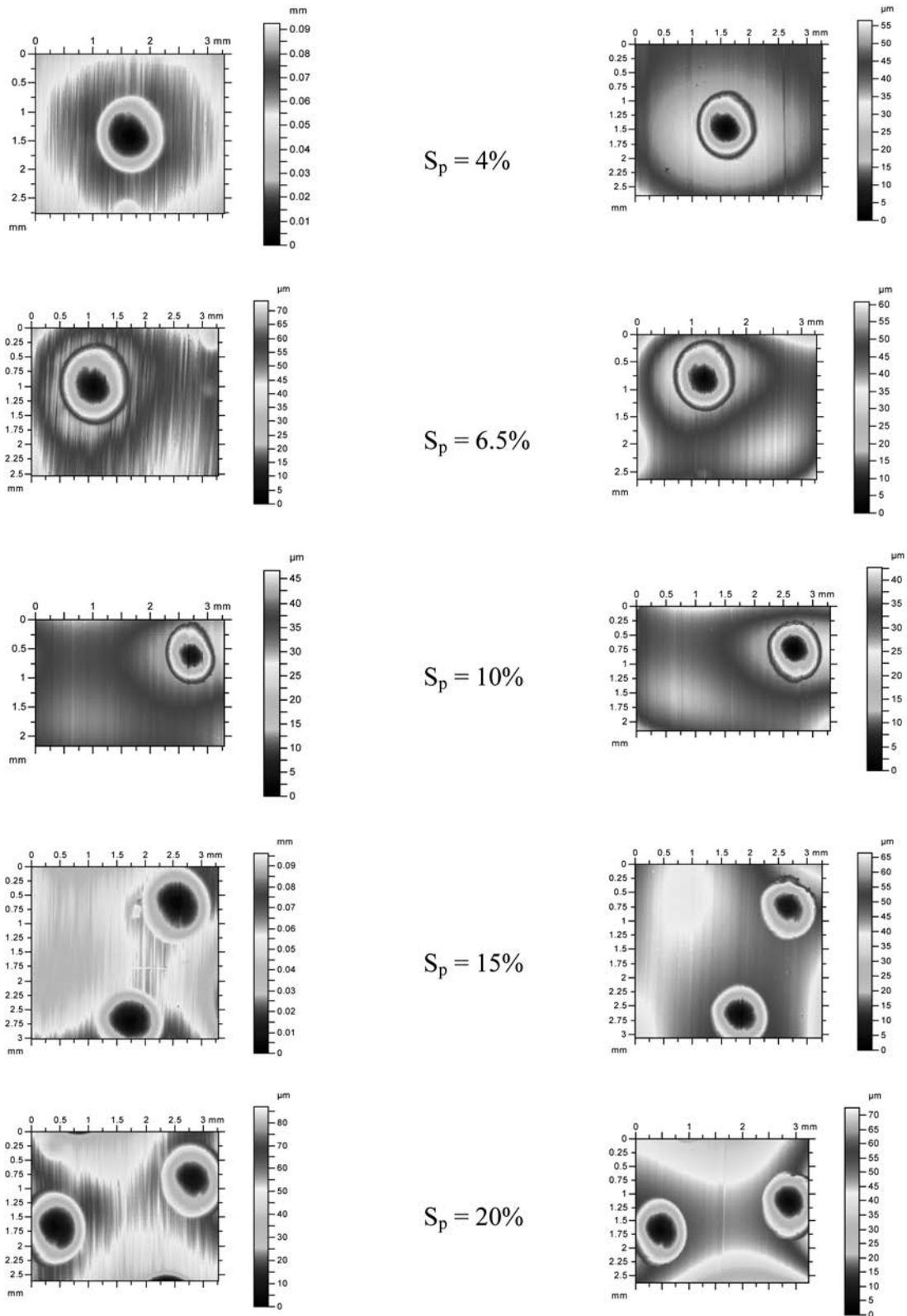
**Fig. 5. Contour plots of textured block samples before (left) and after friction (right)**
