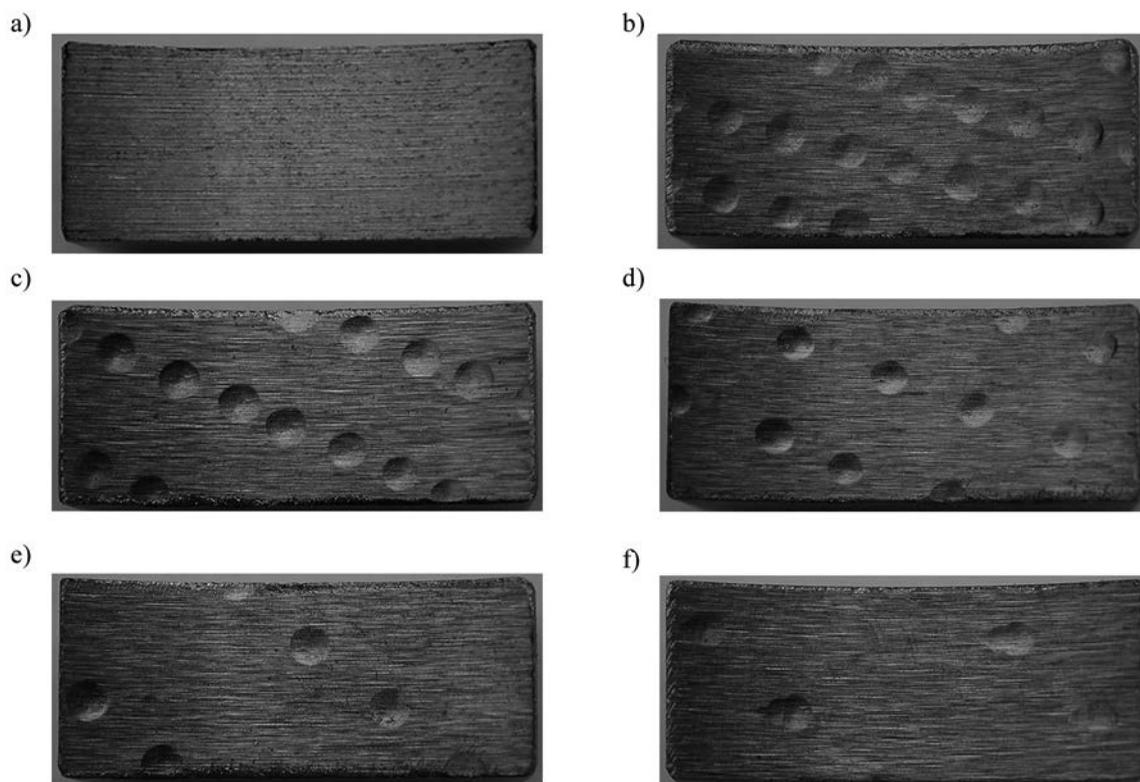
**Fig. 2. Photos of block surfaces before tribologic tests: a) non-textured, b)  $S_p = 20\%$ , c)  $S_p = 15\%$ , d)  $S_p = 10\%$ , e)  $S_p = 6.5\%$ , f)  $S_p = 4\%$**
