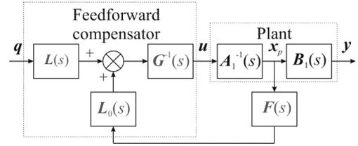
Fig. 1. Structure of the decoupled control system
